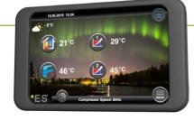
New user-friendly touch screen interface The interface enables quick adjustment of all temperature settings directly from the front page. The software also supports variable temperature settings (curve) for both heating and cooling.
